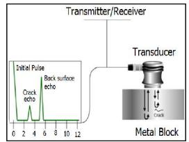
• If there are no flaws in the specimen, output of CRO screen shows normal peaks. If there is any flaw present inside the specimen then CRO screen shows small peaks corresponding to the reflection of ultrasonic waves from flaw.
