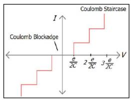
electrons are transferred when the voltage is  $\pm e/2C$ . The repeated tunneling of single electron produces '**Coulomb staircase**'.
