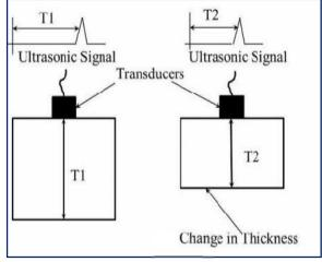
can be calculated using the relation, thickness of the object =  $\frac{vt}{2}$
