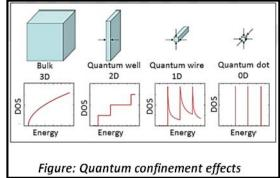
(i) Upon reaching quantum confinement at nanoscale energy levels of nanoparticles become discrete (as shown in the figure). This increases or widens up the band gap and the band gap energy. This results into change in the properties of material at nanoscale.
